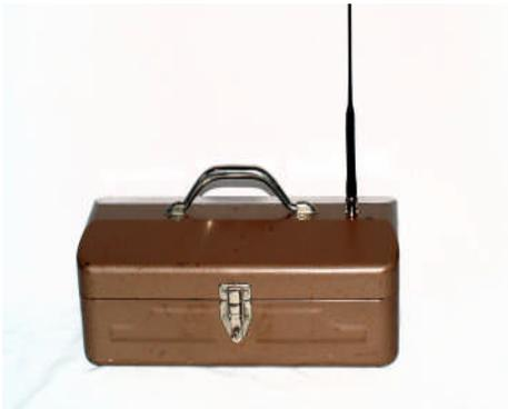
Most guys house the radio and controller, etc., in a old military ammunition case to protect the radio and the controller out in the field. Instead, I follow good old ham radio tradition, and use an old metal toolbox that was just lying about the workshop for cost of \$0. This might cost as much as \$10 if one purchases a new toolbox.
